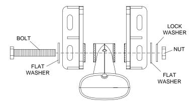
Once you've determined the proper ratchet placement, assemble the transducer and bracket as shown above. Don't tighten the nut at this time.
